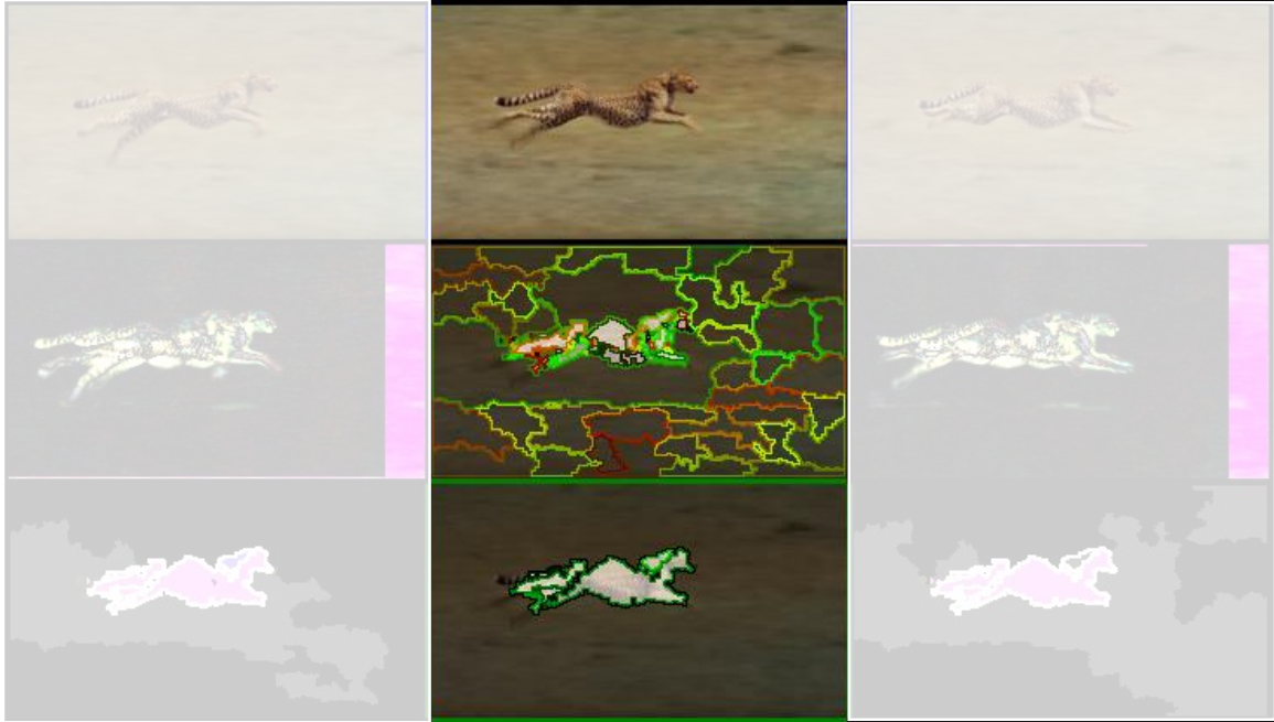
Figure 5-7 Shows the relationship between an original image (top), its segmentation (middle), and its grouping (bottom)
